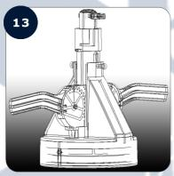
Remove the **Cap** by twisting it counter-clockwise and pulling it **up**.
