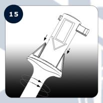
Close the **Front Body (VII)** of the **BIG** by screwing it onto the **Rear Body (I).**
