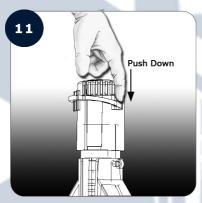
Lower the red clip on the cap's back with your finger until you can insert the Safety Latch (IV).
