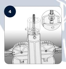
Match the **Piston** (II) to the small **Pin** inside the **Reloading Device.**
