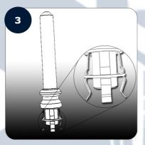
Move the Washer (Ring) (III) on top of the Piston (II) to the small groove on the Needle-Gripping Prongs.
