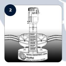
Remove the **cap** at the top of the **Reloading Device**. Twisting it counter clockwise and pull it **up**.
