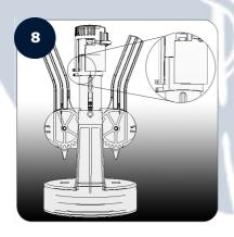
While holding the handles in Position 1, close the cap by pushing it downwards and twisting it clockwise until the two red string holders match.
