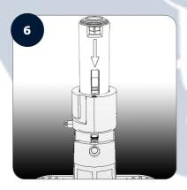
Slide the Rear Body of the B.I.G. (I) over the Piston (II) and Spring (IV); make sure that the Bolder Raised Arrow matches the groove on the back of the device and the Shallower Arrow is pointing at the red line on the front of the device.
